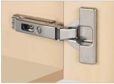
The hinges are particularly suitable for door thicknesses from 10 mm and above. Note drilling depth for hinge cup 8.0 mm.
