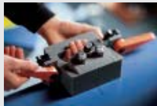
Position drilling jig and tighten
