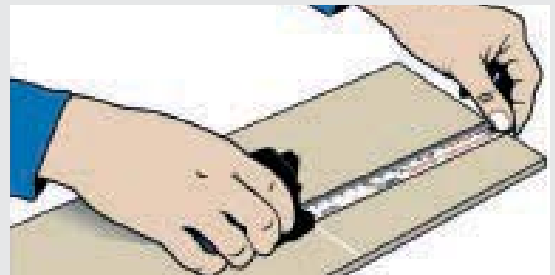
Transferring the measurement onto the workpiece
