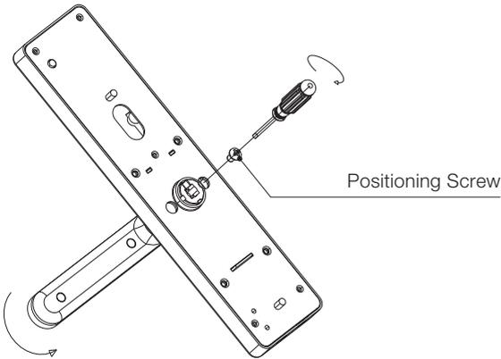
1. Loosen positioning screw
