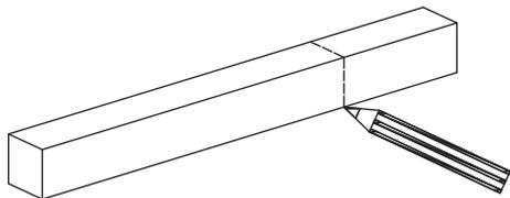
1. Use below template and mark a cutting line on the spindle according to the door thickness.
