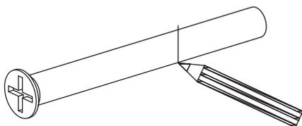
1. Use below template and mark a cutting line on the Screw according to the door thickness.
