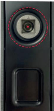
1. Loosen the screw in the red mark, until handle is movable.
