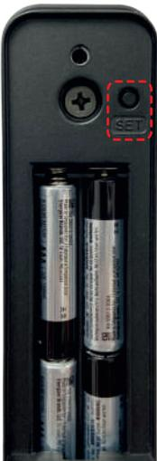
Open the battery cover then press the 'set' button for 5 seconds until hear the voice "Beep Beep".
