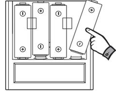
When the battery voltage gets downed, it's the battery exchange time. The saved melody ring comes out every locked and unlocked time.
