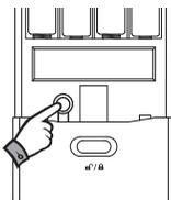
Open the battery cover and press [ INPUT BUTTON ]
