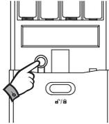
Open the battery cover and press [ INPUT BUTTON ] shortly (one short beep sound)
