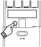
Open the battery cover and press [ INPUT BUTTON ] shortly (two short beep sound)
