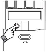
Open the battery cover and press [ INPUT BUTTON ] shortly (two short beep sound)
