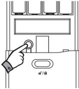
Open battery cover and press [ INPUT BUTTON ] shortly (one short beep sound)
