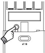
Open battery cover and press [ INPUT BUTTON ] shortly (one short beep sound)
