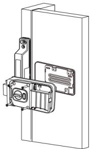
6. Insert 4 x AA batteries and fix batteries cover screw.
