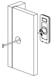
2. Get the external module cable through the internal module bracket and fix screws from inside of the door.
