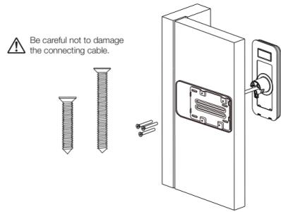
3. Depending on installation condition, fix proper position of striker with screws.
