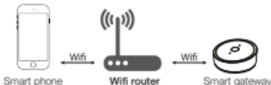
Ensure the smart switch is within wireless range of the Gateway to ensure a successful connection between the switch and the gateway.
